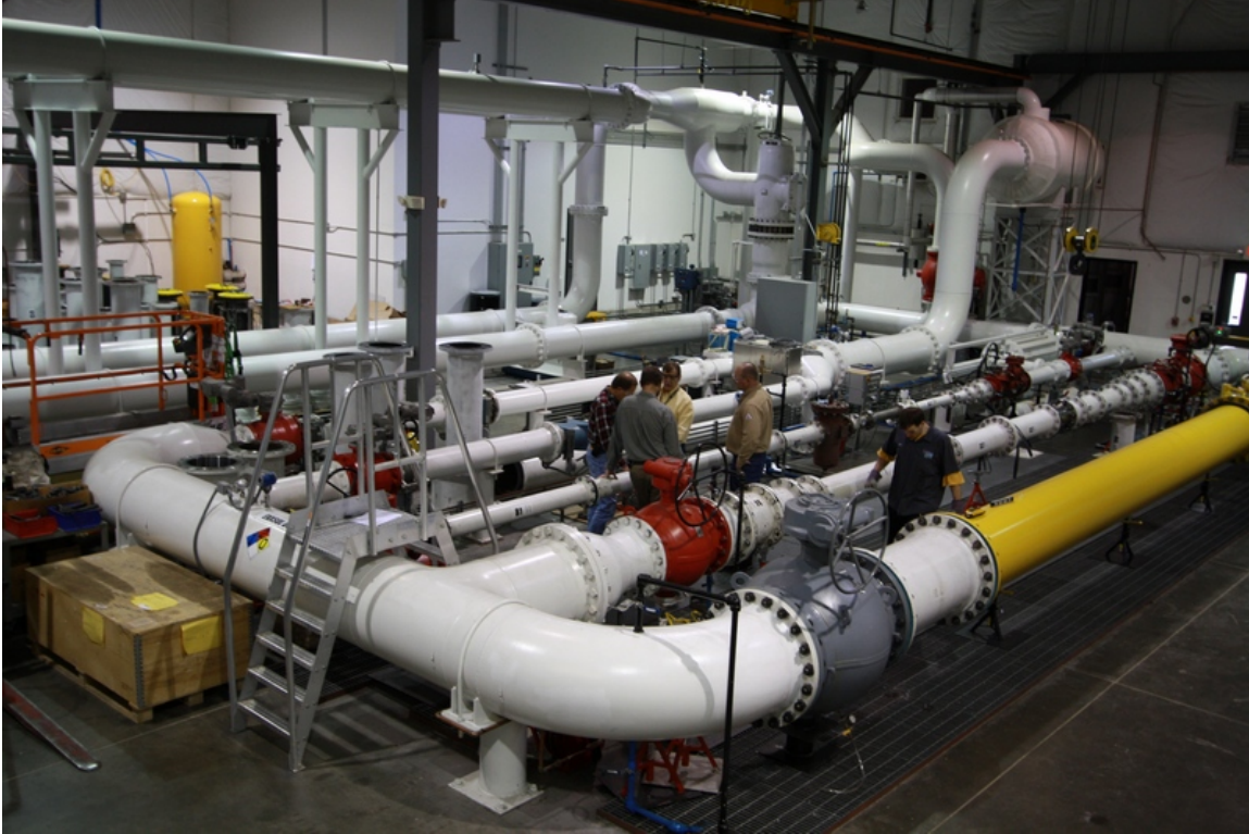
Figure 1B—Alternate Test Meter Run Configuration
